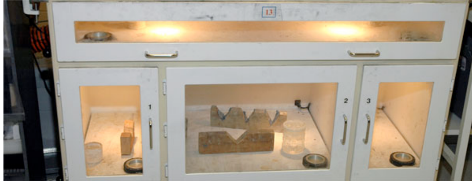
A chamber specially designed for exposing latent prints to super glue fumes. (Courtesy of Scott Campbell, Ron Smith & Associates)
